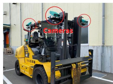
Intelligent cameras installed on forklifts
