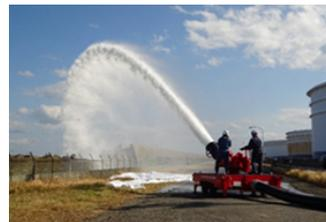
High-capacity foam water canon (Oita Refinery)
