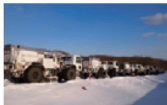
Vibration trucks performing seismic work
