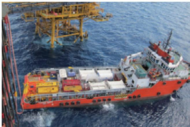
A supply vessel provides CO<sub>2</sub> for injection into the reservoir.
