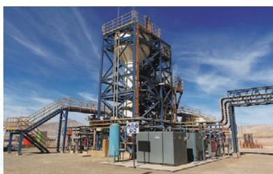
Bioreactor (microorganism culture equipment) established at Radomiro Tomic mine
