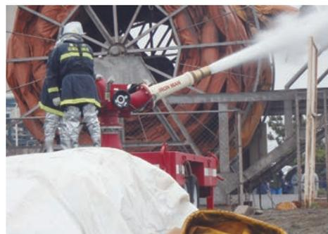
Water discharge drill using a high-capacity sprayer
