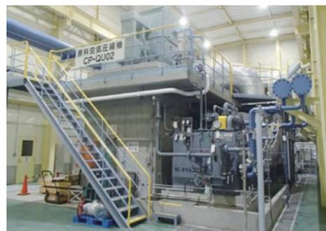
Equipment for compressing the air used to make oxygen
