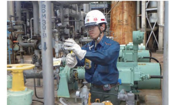
Employee testing for exposure using individual samplers
