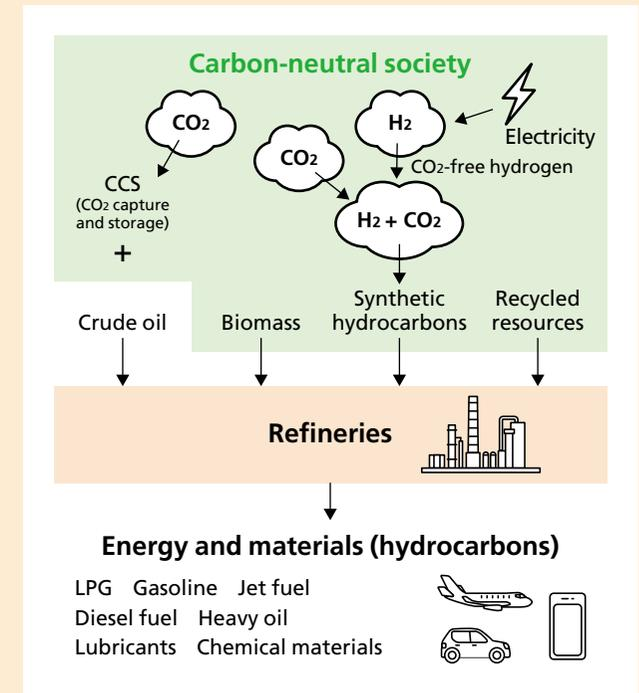
In a carbon-neutral society, refineries will produce energy and materials from raw materials that do not increase CO<sub>2</sub> in the atmosphere, such as biomass, synthetic hydrocarbons produced from hydrogen and CO<sub>2</sub>, and recycled resources. Conventional crude oil processing will be combined with CCS to achieve net zero CO<sub>2</sub> emissions.
