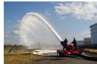
High-capacity foam water canon (Oita Refinery)
