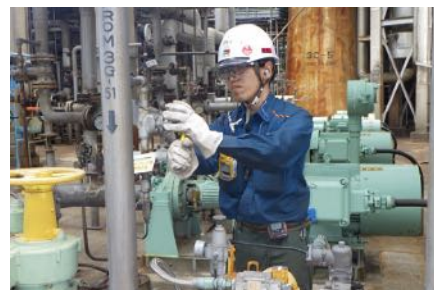
Employee testing for exposure to chemical substances using individual samplers
