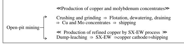
Notes 1: (1)Dump-leaching means a process to extract (leach) copper by sprinkling sulfuric acid over a pile of uncrushed copper ore.
