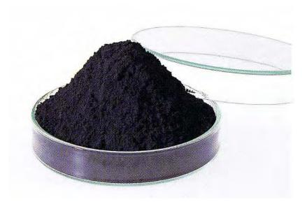
Cathode materials for automotive lithium-ion batteries
