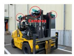
Intelligent cameras installed on forklifts
