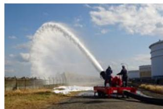
High-capacity foam water canon (Oita Refinery)
