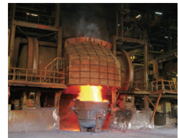
Converter in use in the recycling process at Saganoseki Smelter & Refinery
