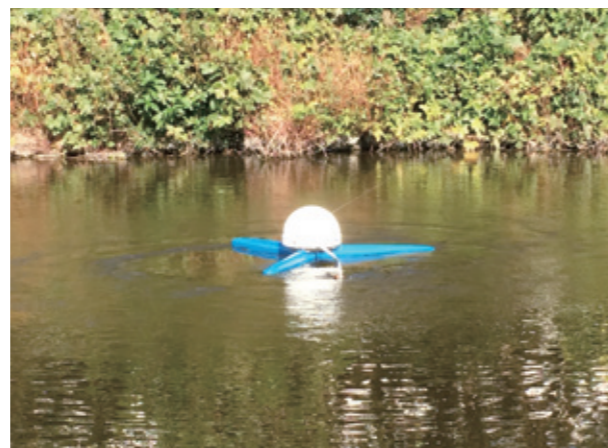
Biofan installed to keep pond water clean
