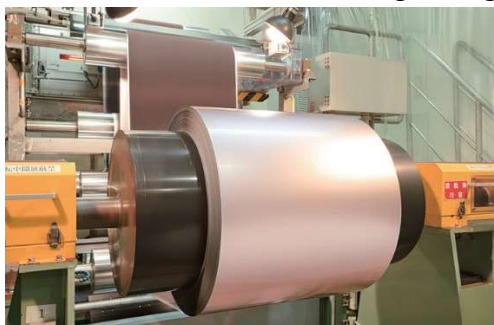
Processing of treated rolled copper surface (Hitachi Works)
